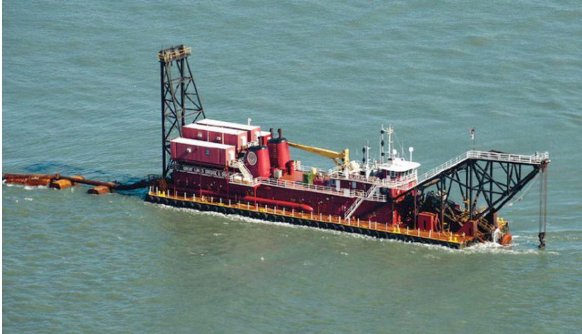
Photo Caption: Cutter Suction Dredge 'Alaska' previously delivered by Conrad to Great Lakes Dredge & Dock
