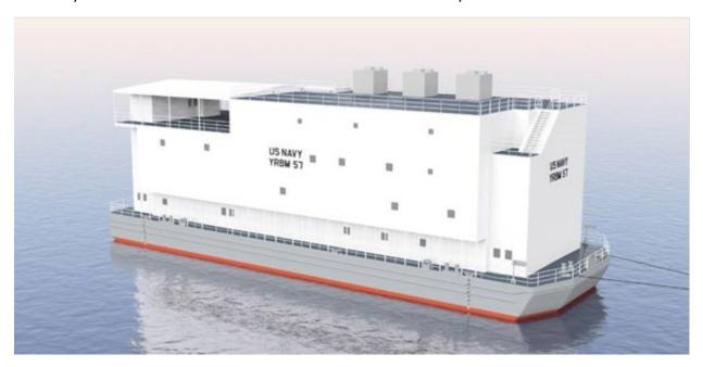
The YRBM barge is an ABS A1 Accommodation Barge with a 151'-4" x 49'-4" x 14' footprint. The vessel provides pier side living accommodations capable of berthing 199 mixed gender personnel, messing for
