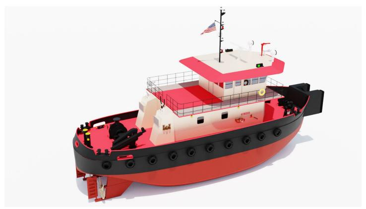
The CELRE Detroit Ice Class Tugboats measure 76' x 25' x 10'-8.5" and are ABS classed as Maltese Cross A-1 Towing Vessels, Ice Class C0, Great Lakes Service with Maltese Cross AMS. Each vessel shall also comply with USCG 46 CFR SubChapter M requirements. The tugs are diesel powered, twin screw, open wheel, with 1,600 BHP and have deckhouses with galley/mess, berths, and sanitary facilities for a crew of 3.
