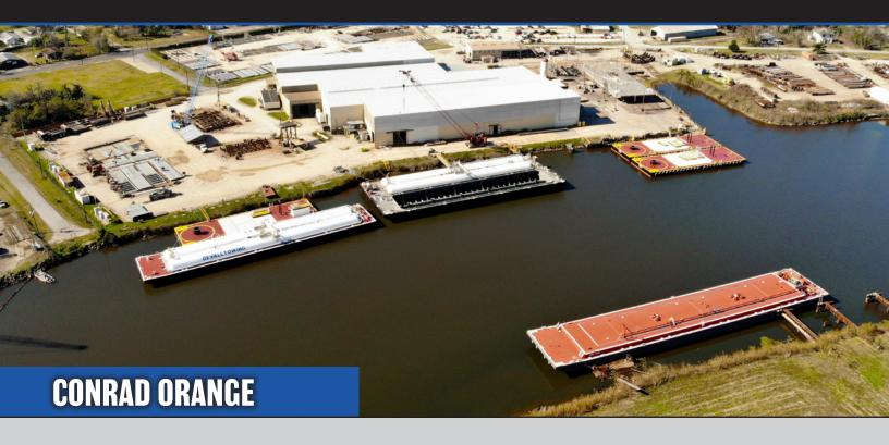
Conrad Orange is located on 24-Acres on the Sabine River, just north of the Gulf Intracoastal Waterway in Orange, Texas and is purpose-designed for vessel construction efficiency. The shippard has six construction bays with approximately 115,000 square feet of enclosed area, allowing work to be continued without weather delays. Conrad Orange has built a wide variety of vessels for commercial and government markets.
